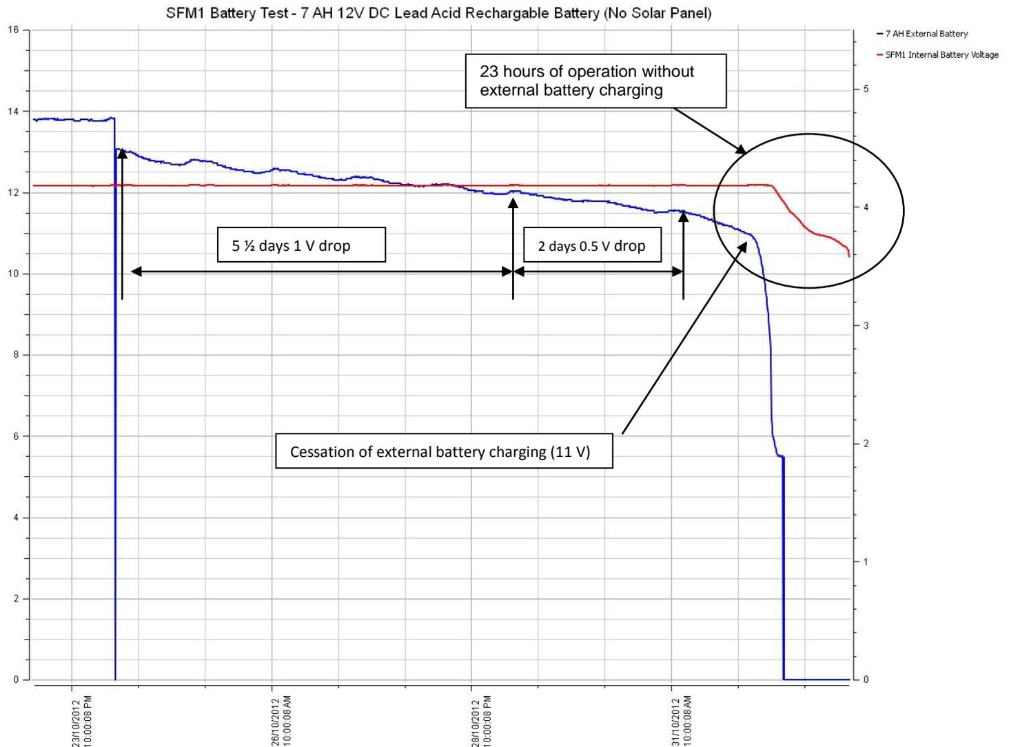
Figure 4. SFM1 Internal battery voltage overlaid against external 7 Ah battery voltage
