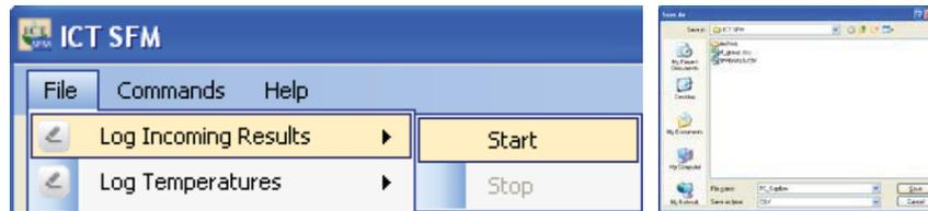
Figure 101 the Menu sequence required to start Logging Incoming Sap Flow data direct to the computer
